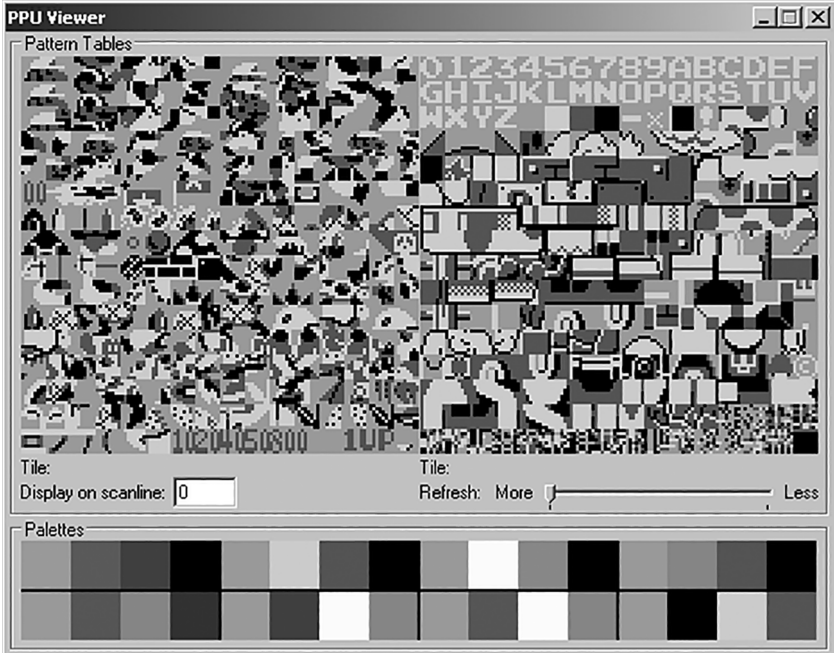
1.5 The contents of Super Mario Bros. 's CHR-ROM. Each pattern table contains 256 8x8 tiles. In Super Mario Bros. , pattern table 0 (left) contains sprites and pattern table 1 (right) contains background tiles. (Emulator: FCEUX 2.1.5)
