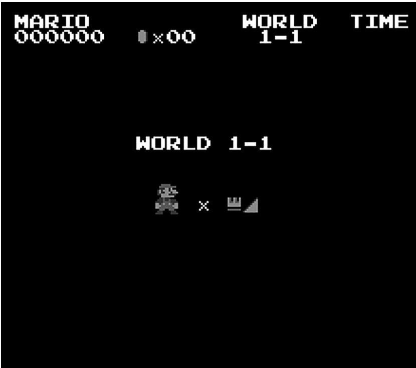
4.9 Accumulating more than nine lives in Super Mario Bros. causes unintended CHR-ROM tiles to seep into the lives counter. (Emulator: Macifom 0.16)
