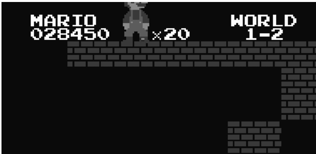
4.6 The PPU's tile priority rules reveal sprite o's location without disabling background tile visibility. (Emulator: FCEUX 2.1.5)
