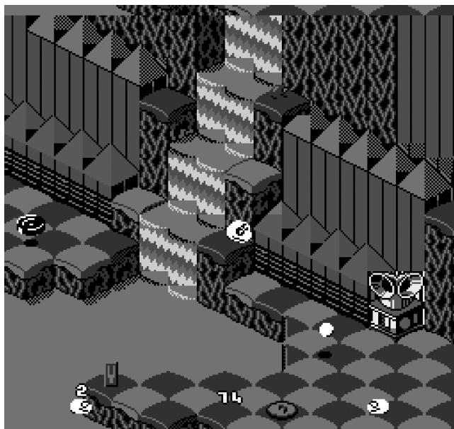
1.6 A screenshot from Snake Rattle N Roll shows abrupt color changes across background attribute boundaries, especially among the pyramids and waterfalls. (Emulator: Macifom o.16)
