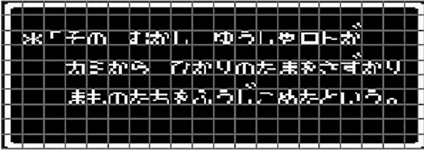
6.5 An enlarged screenshot from an emulator VRAM Viewer shows the name table distribution of hiragana characters in Dragon Quest 's dialogue box. Note that diacritics occupy their own tiles in separate rows above the primary characters. (Emulator: NO$NES v1.0)
