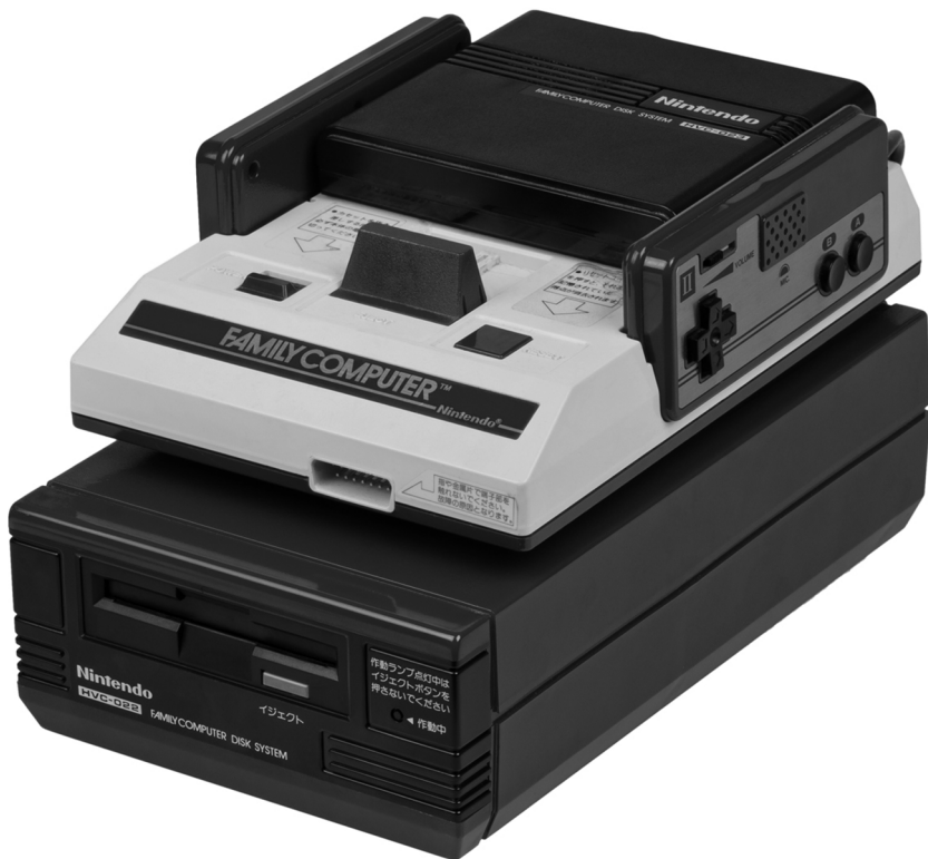
5.1 A Famicom sitting atop the Family Computer Disk System peripheral. The black RAM adapter is attached to the Famicom's cartridge slot. (Source: Evan Amos, Wikimedia Commons)
