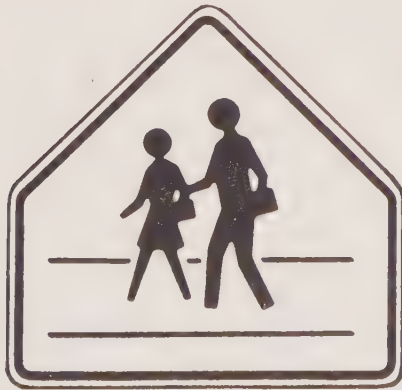
7.4 · School crossing sign.
